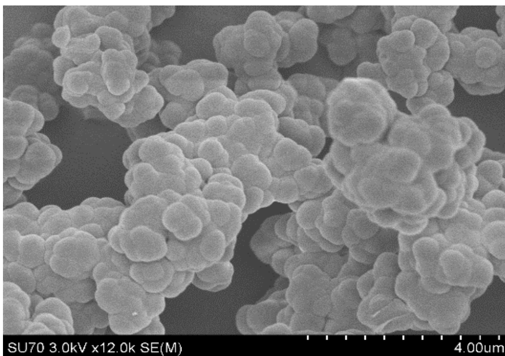
Figure 4.4. Scanning Electron Microscopy (SEM) Imaging of DBLP-4: A sample DBLP-4 was prepared by dispersing the material onto a sticky carbon surface attached to a flat aluminum sample holder. The sample was then gold coated using an EMS (Electron Microscopy Sciences) 550x Sputter Coater at 1 \times 10^{-1} mbar of pressure in a nitrogen atmosphere for 90 seconds while maintaining 20 mA of current.
