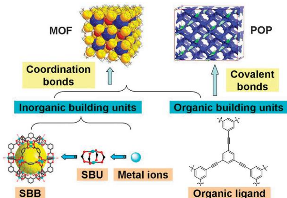
Figure 1.4: Representation of a typical MOF and POP. Adapted from Ref. 6 with permission from The Royal Society of Chemistry.
